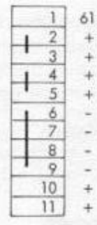
Terminal Strip Allocation
